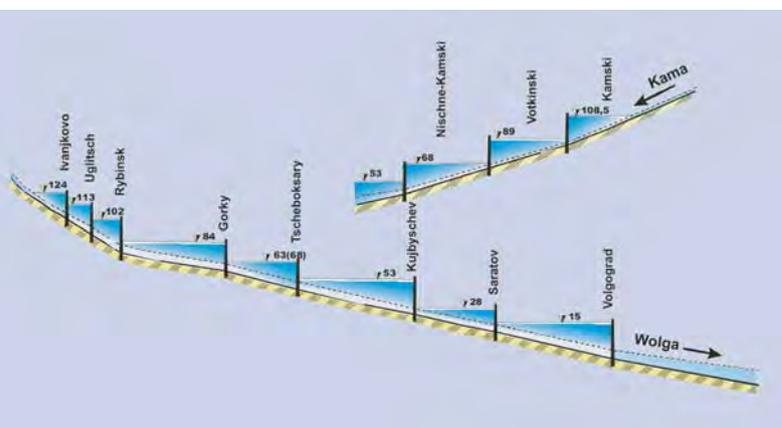
Longitudinal section of the Volga and Kama barrage chain
