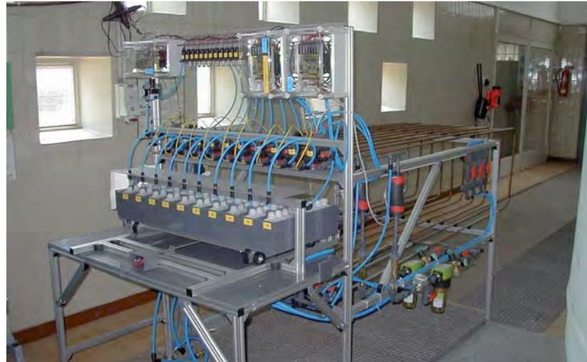
Transportable test rig for assessing the influence of water quality on corrosion on site
