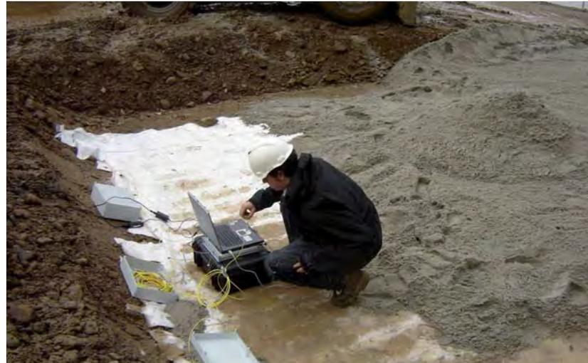
Controlled measuring on an area of sensor-based geotextile as part of the application process: field test in Swienna Poremba (Poland)
