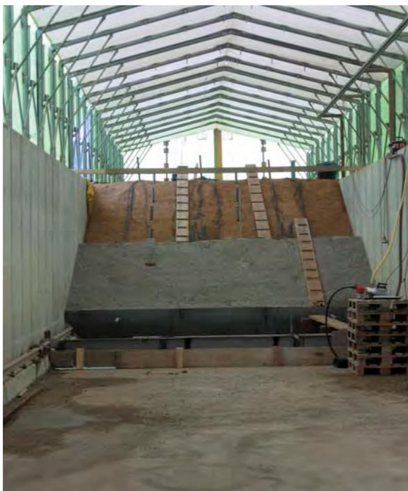
The model dyke on a natural scale (height: 3 m) proved the technical feasibility of the stabilisation procedure (viewed from land side)
